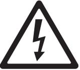
**Important!** Do not insert or remove live Neutrik PowerCon connectors to apply or cut power, as this may cause arcing at the terminals and damage the connectors.
